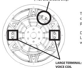
The Elite.12 has three terminals. The two larger terminals are connected to the voice coils. The small terminal is used to power the LEDs with a +12v and ground connection only.
